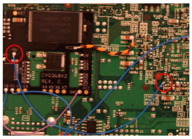
As an alternative to the RB cable you can scratch off the RB point on the mainboard as described in the chapter 2.1
