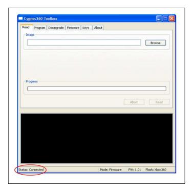
Now that you have established the connection between the toolbox and Cygnos360 V2 you can start to read flash, program the flash or program Cygnos360 V2 with a new firmware.
