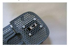
Make sure you cut the hole exactly as in the pictures here, otherwise you might hit some plastic parts on the front which will hinder you from closing the part while the Cygnos V2 USB board is installed.
