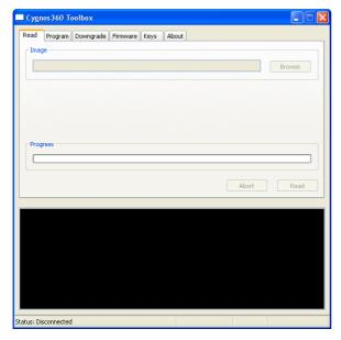
As soon as you plug in your USB cable and connect it to Cygnos360 V2 the toolbox will recognize it and show the status "connected" as well as the currently selected NAND flash. (either Cygnos NAND or Xbox360 NAND). If you flip the switch you can see that the selection of the flash memory changes. When the LED is lit in blue the toolbox should show "Cygnos NAND" if it is not lit it should be "Xbox360 NAND".
